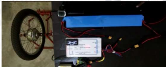
Initial Hardware and Software testing of Duo pack board 350W hub motor
